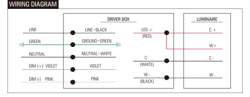
UP / DOWN LINEAR LED LUMINAIRE INSTALLATION INSTRUCTIONS
